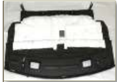
COVERING SHELF Ø3.2 BLIND RIVET
